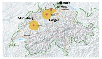
Planning zone 1 with radius 3 to 5 km and zone 2 with radius of 20 km is divided into 6 overlapping sectors of 120 degrees (on Swiss territory). The planning zone for the predistribution of stable iodine is 50 km. In case of emergency, iodine can be distributed to the population outside the 50 km zone within 12 hours.
