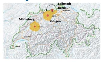
Planning zone 1 with radius 3 to 5 km and zone 2 with radius of 20 km is divided into 6 overlapping sectors of 120 degrees (on Swiss territory). The planning zone for the predistribution of stable iodine is 50 km. In case of emergency, iodine can be distributed to the population outside the 50 km zone within 12 hours.
